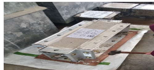
Figure 4: Mould with concrete admixture sampling
