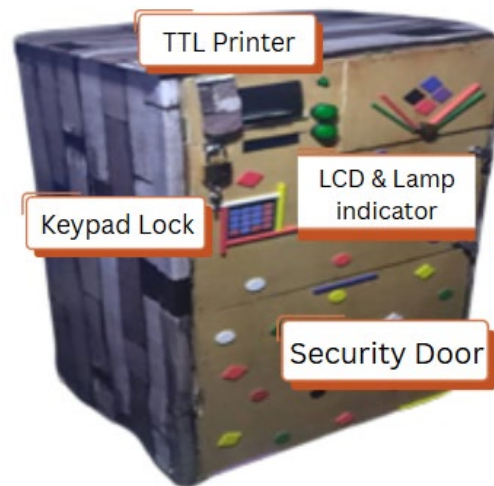
Figure 3: S-Parcel Mailbox With Printed Delivery Receipt prototype
